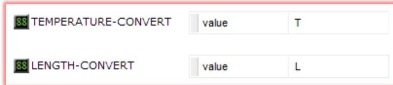
This indicates that in-type can have one of two values, T for temperature or L for length. The copybook also indicates that the temperature area redefines the length area, which means that you can only have one or the other, and the value of in-type determines which of those it is.
